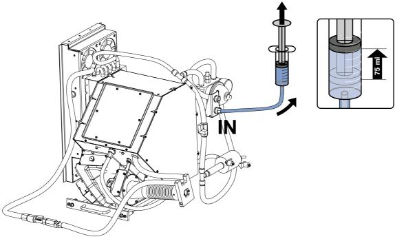
Image 2-18 Calibrate cooling circuit
